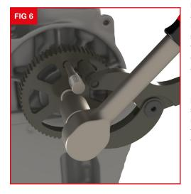
Once the reaction bolt B bottoms out in the camshaft remove it and complete the fitment using the OEM fixing bolt.
