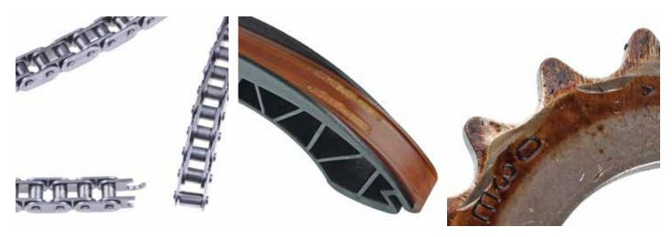
As vehicle engines develop with a reduction in weight and capacity and an increase in power output. Increased stresses are put on these linking components, particularly in high powered, fuel efficient diesel and direct injection petrol engines. Coupled with other emission reducing technologies, such as stop-start and hybrid vehicles there is a need to minimise timing chain wear as vehicle emission legislation continues to tighten.
