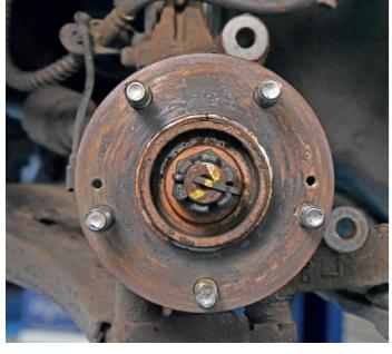
Brake disc ,run-out' must be checked with a dial gauge (Fig 2) with the brake disc secured to the hub, taking note of the point of maximum variation. The utmost recommended ,run-out' is 0.10mm - however, this number may be lower subject to the vehicle manufacturer's specification.
