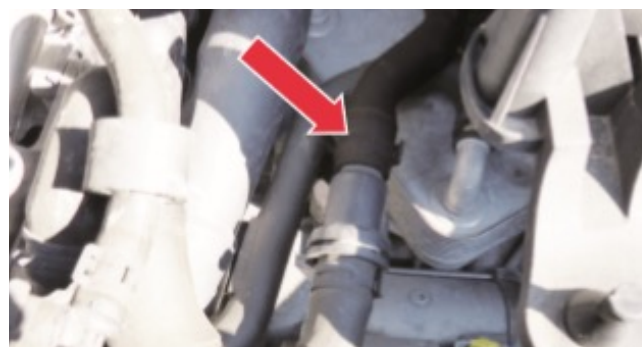
Fig 1: The thermostat is integrated into the flexible hose at the heat exchanger (under the air filter housing).
