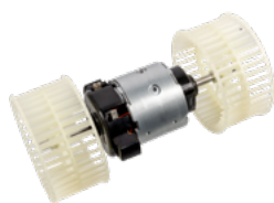
febi 43775 Interior Fan Assembly with motor to fit Actros II+III Repl. no. 003 830 05 08
