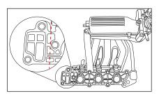
Once removed from the car, hold or carefully clamp the plastic inlet manifold. Mark the coolant blanking section of the manifold that you are about to saw through, making sure that you mark a section slightly larger than the size of the new blanking plate. This is to ensure there is no interference between the manifold and new blanking plate when they are fitted to the engine. Measure twice - cut once!
