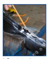
4. To protect against corrosion it is necessary to cover the exposed bare metal. Apply a layer of primer to the bare metal. Then once dry, apply a coating of an oil based paint. Alternatively use a good quality stone-chip guard type paint.
