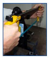
2. Using a hacksaw, cut through the bracket vertically as close to the welded flange as possible.
