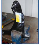
3. Using a file or hand grinder, remove any burrs or sharp edges.
