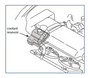
**Note:** Care is required when removing the coolant hose shown in the picture below, in order to avoid damage to the outlet on the radiator.
